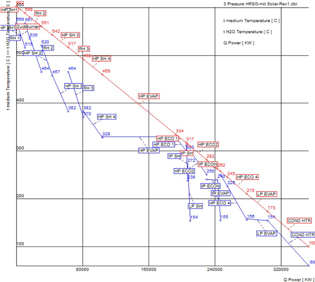
Pic [5] A typical conventional HRSG configuration in Q- T diagram
