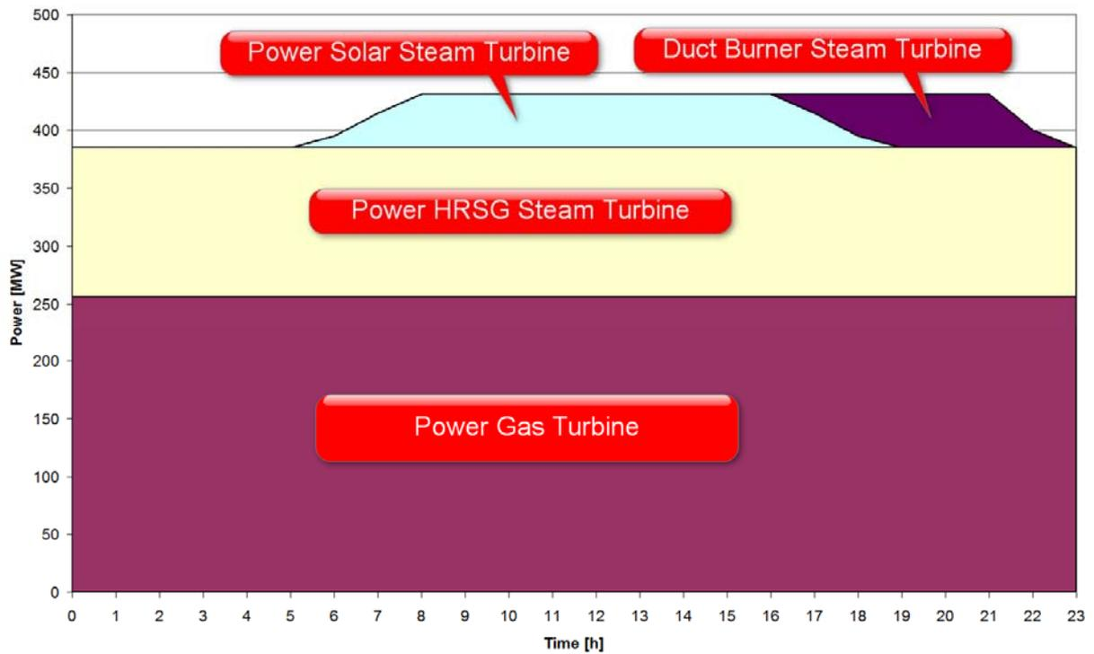
Pic [9] Time vs. power of ISCCS plant
