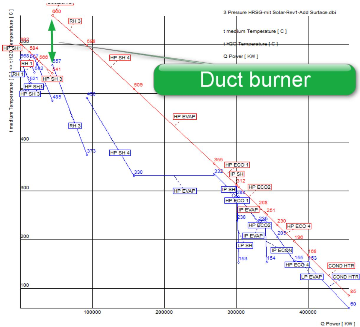
Pic [7] Q-T diagram duct burner mode
