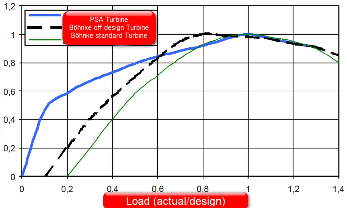
Pic [8] Steam turbine load vs. relative efficiency to design point efficiency
